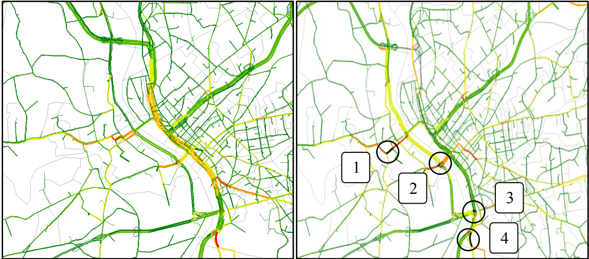
Figure 7 Change in the congestion from a normal day to the chemical spill.
